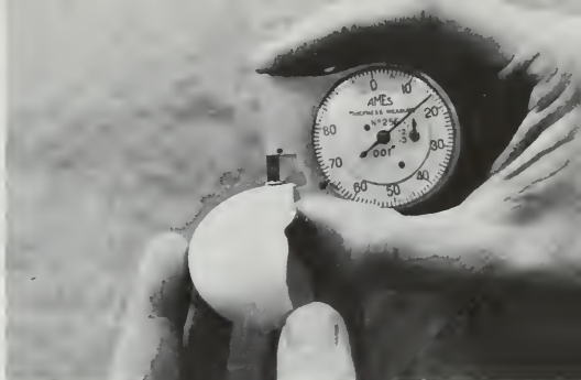
The thickness of shells is measured as part of the work of developing strains that will lay eggs whose shells are strong enough to withstand handling in marketing.
